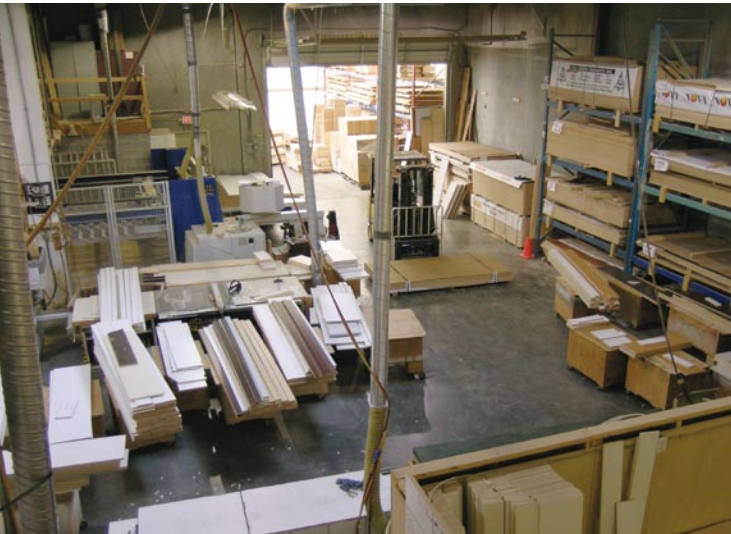
These before and after views highlight the changes in the machining area. With the new machinery purchases and other equipment repositioned, material now moves quickly and efficiently from the Schelling and Holz-Her panel saws to the Biesse Rover machining center and on to the IMA single-sided edgebander or Biesse/Polymac radius edgebander, with no buildup of work in process.
