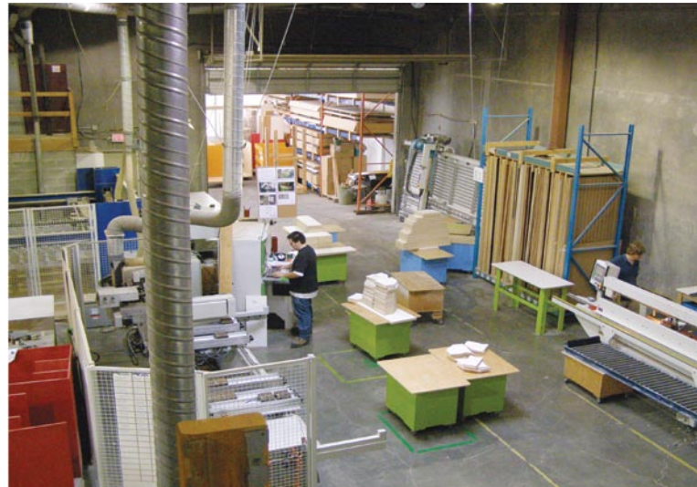
These before and after views highlight the changes in the machining area. With the new machinery purchases and other equipment repositioned, material now moves quickly and efficiently from the Schelling and Holz-Her panel saws to the Biesse Rover machining center and on to the IMA single-sided edgebander or Biesse/Polymac radius edgebander, with no buildup of work in process.
