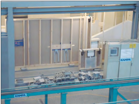
Preinstalled plumbing components
